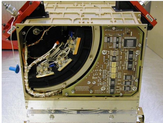
FIG. 22 The flight model of the NPD sensor during installation.
